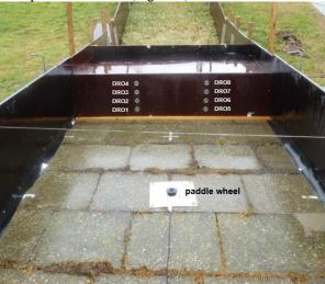
Figure 9. Pressure sensors in the step.
