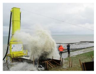
Figure 7. Wave impulse with the wave run-up simulator
